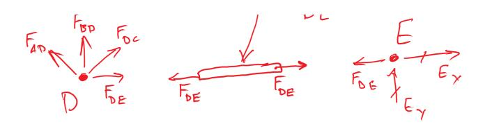
We will determine the force in each member of the truss and indicate whether the members are in tension or compression.
