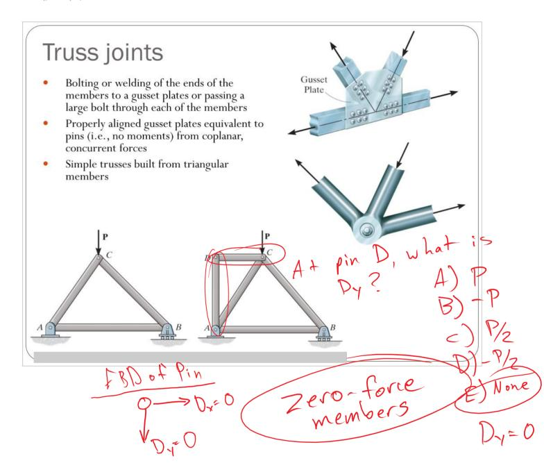
Method of joints or, method of pins
