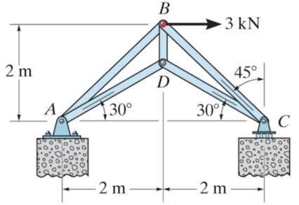
We will determine the force in each member of the truss and indicate whether the members are in tension or compression.
