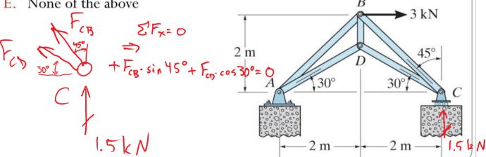
We will determine the force in each member of the truss and indicate whether the members are in tension or compression.
